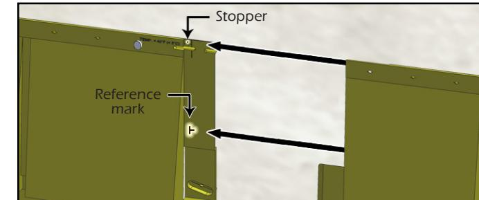
Installation when outdoor temperature is below 40°F(5°C), stop at the temperature line.
