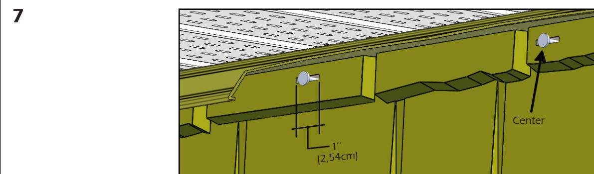
If you need to attach the siding in an area other than the installation hole, create a 1"(2,54 cm) long slot to allow nailing. Always nail in the middle of the slot.
